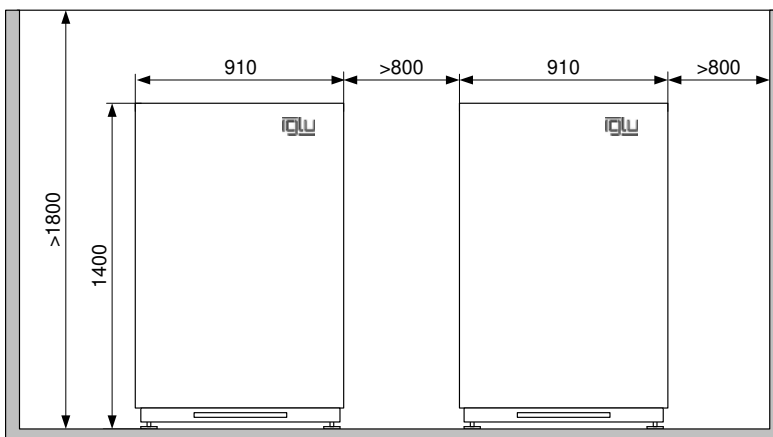
Front view: 2 heat pumps
