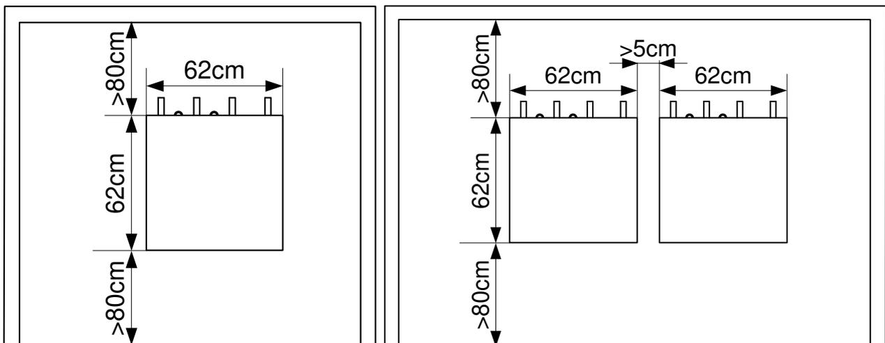
Heat pump with integrated water tank dimensions and connection nozzles
