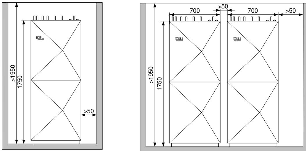
Design dimensions of the heat pump from the top
