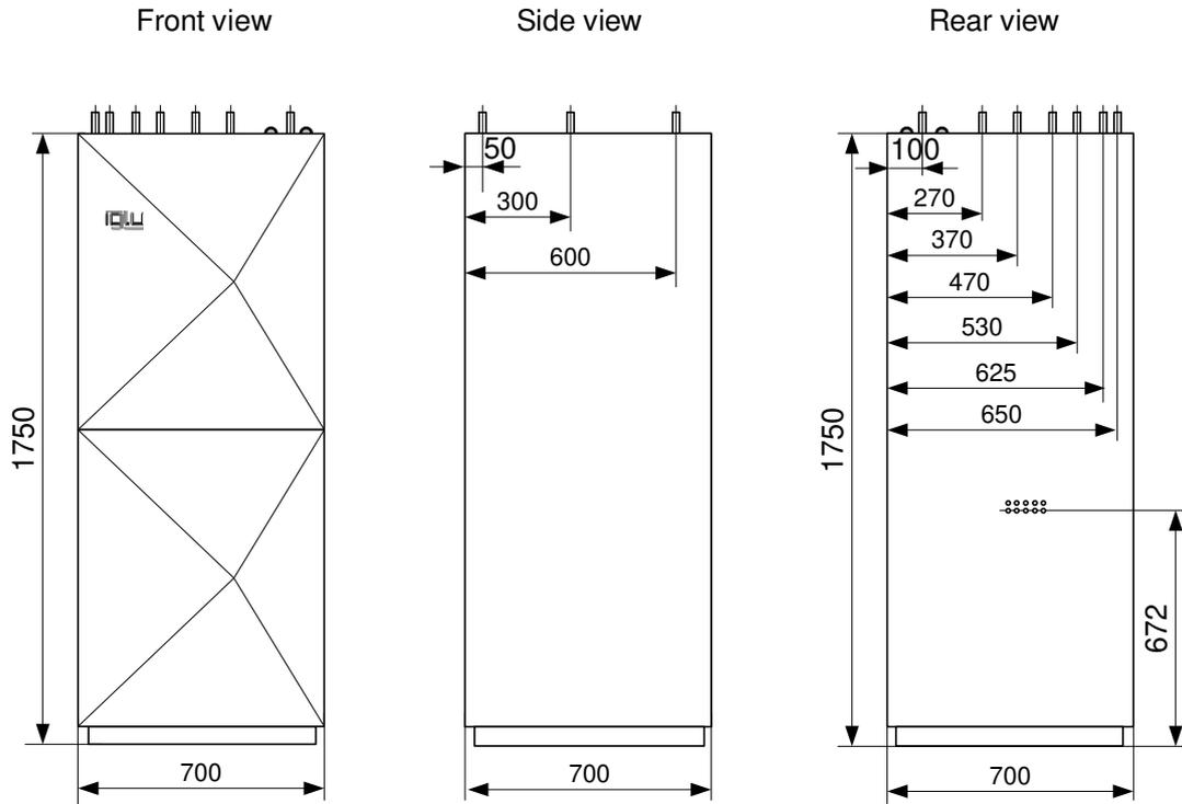
Design dimensions of the heat pump with integrated water tank from the front
